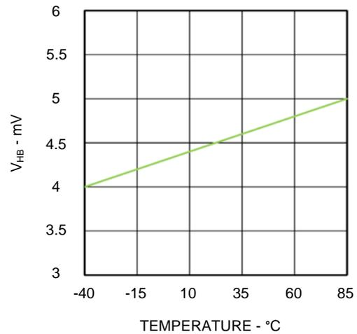
TSM9117/9118 Reference Voltage vs Temperature
