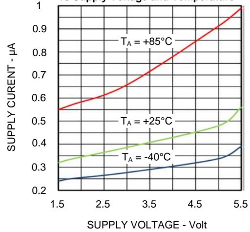
**TSM9117/9118 Supply Current vs Temperature**
