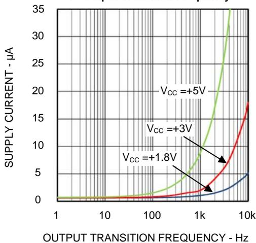
**TSM9119/9120 Supply Current vs Output Transition Frequency**
