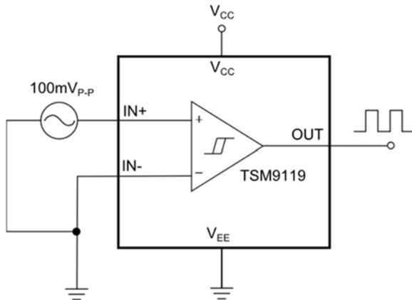
**Figure 5:** A Simple Zero-Crossing Detector
