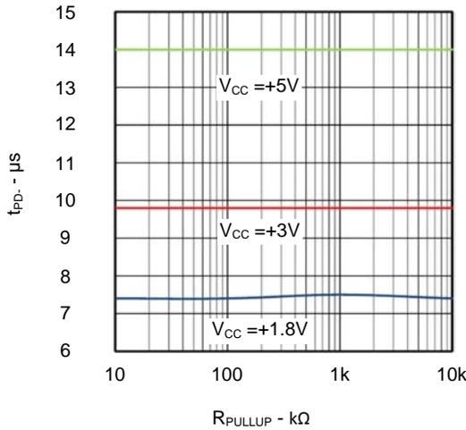
TSM9118/9120 Propagation Delay ( $t_{PD+}$ ) vs Pullup Resistance
