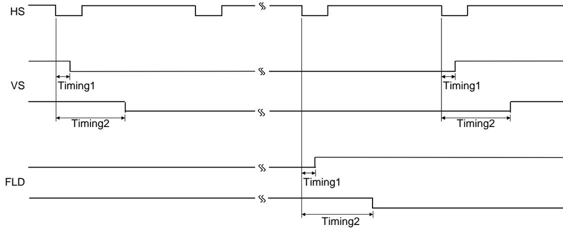
Timing1 : 40 system clock(54MHz) for the Even field with VSMODE=1 or Odd field
