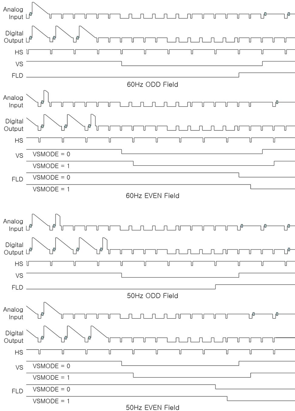
Fig11 Vertical Timing for 60Hz / 50Hz Video
